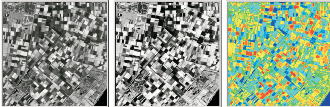
Figure 10.8: Single band of a Landsat TM image of a polder area in The Netherlands. Image without contrast enhancement (left); histogram equalization (middle) and pseudo-colour representation (right).
