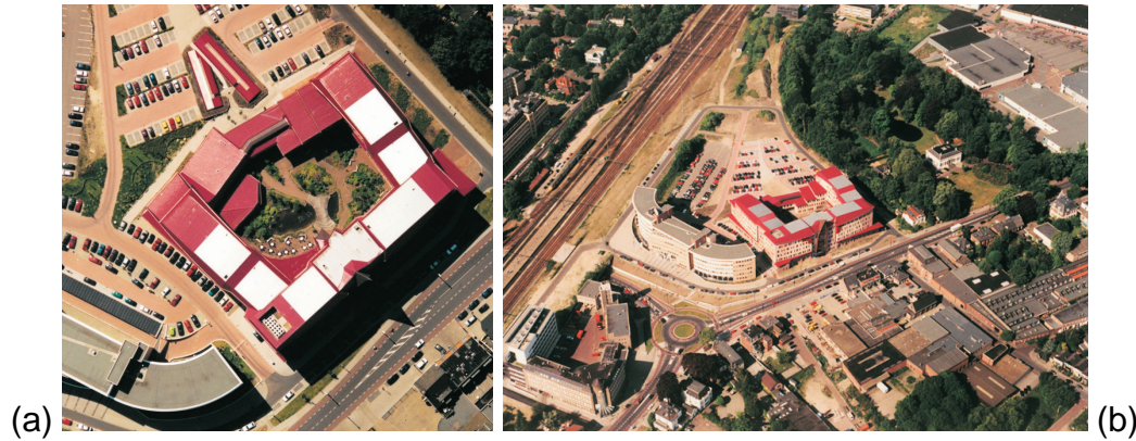
Figure 4.2: Vertical (a) and oblique (b) aerial photo of the ITC building. Photos by Paul Hofstee, 1999.
