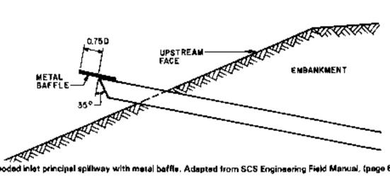
Hooded inlet principal splitway with metal baffle. Adapted from SCS Engineering Field Manual, (page 6-49)
