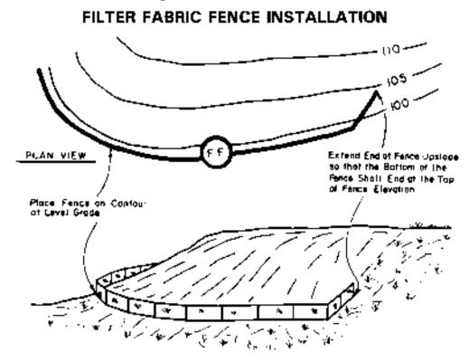
Figure 2-3 : Filter Fabric Fence Installation
