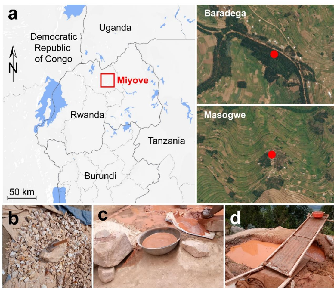
Figure 1. Artisanal gold mining. (a) The location of the Miyove gold mine and landscape of two sampling sites (red points). The photos of three artisanal gold mining methods at Miyove: (b) gold ore breaking with Hammer; (c) African stone grinding mill; (d) old-style table shaking system.
