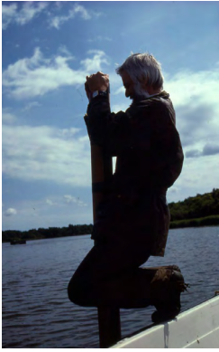
Fig. 6.1 The author thrusting a plastic drainpipe into the sediments of a shallow lake to obtain a core. The pipe had previously been cut longitudinally and then re-taped together with strong waterproof tape that could be cut on land to retrieve the sediment. An intact tube can be used but then a plunger is needed to push the sediment out of the core. Modern attitudes to health and safety now mandate the wearing of a life-jacket.
