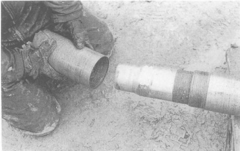
Figure 7. Sedidrill system, Mazier corer, at the site of one of the former Bòbila Ordis Early Pleistocene lakes, Spain (photo S. Leroy).
