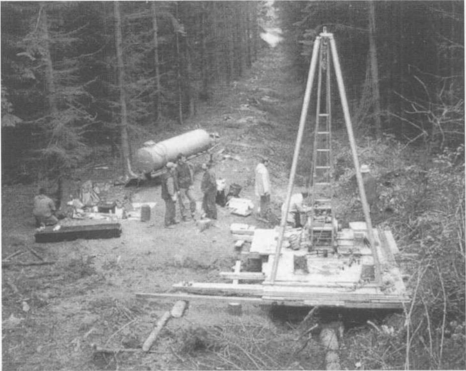
Figure 8. Usinger system being set up on land near one of the Eifel maar lakes in Germany (photo S. Leroy).
