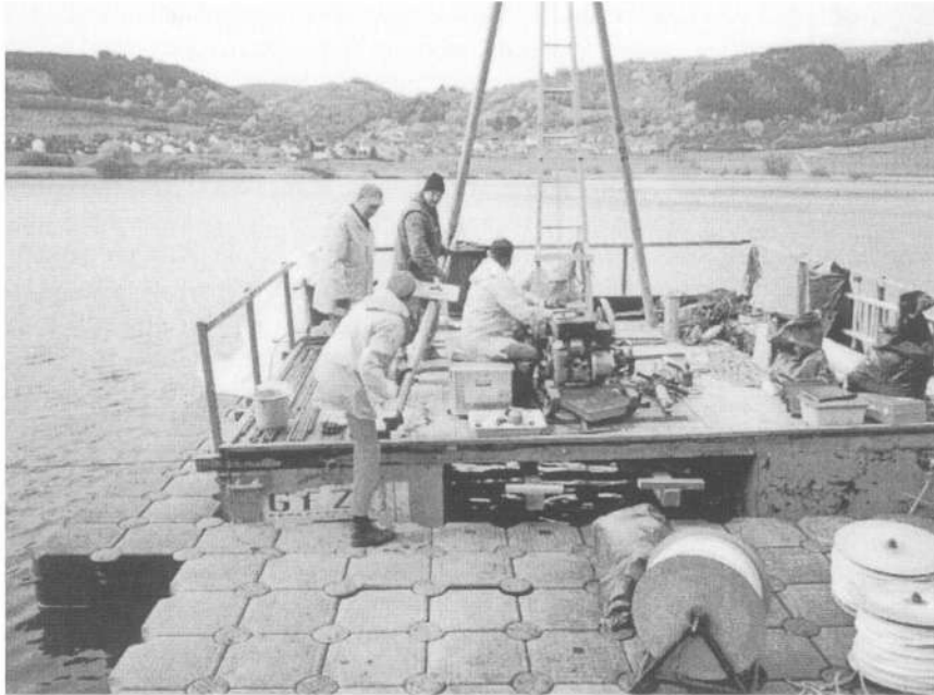
Figure 1. The GeoForschungsZentrum platform system, which uses modular heavy-duty plastic cells, at Meerfeldermaar, Germany (photo A. Brauer).
