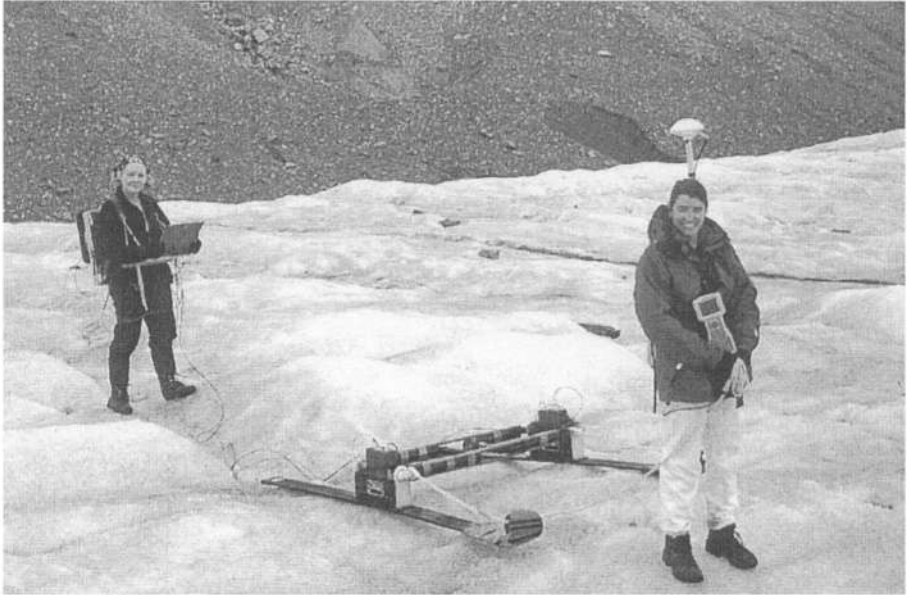
Figure 2. An example of how a GPR can be towed across ice on foot. The person in front is also carrying a differential GPS receiver so that the location of the profiles can be precisely mapped.
