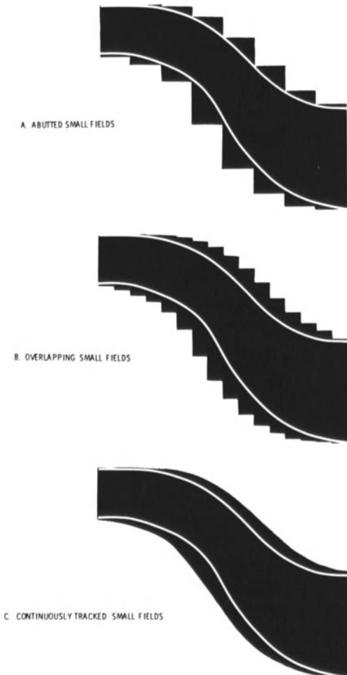
Figure 14. Shaping an irradiated field using a computer-controlled tracking machine. (a) Using abutted small beams. (b) Using overlapping small beams. (c) Using continuously tracked small beams.
