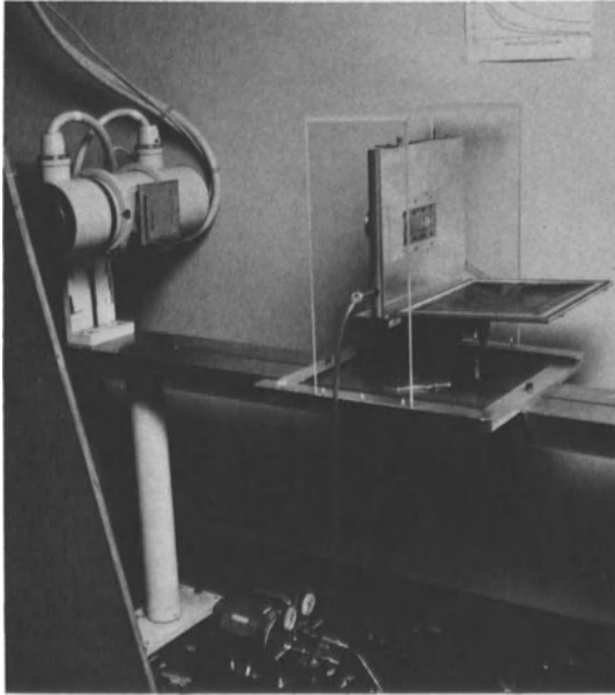
Figure 12. Photograph of the slit device for obtaining slit images on screen-film systems.
