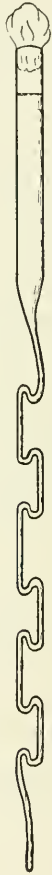
Figure 123. Capillary tube used for the sterilization of Trichomonas hominis . The whole tube is filled with sterile fluid, the lower end sealed in a flame, and the Protozoa to be sterilized are layered on to the fluid at the large end. The Protozoa eventually migrate through the capillary portion, but the associated bacteria are trapped at the first or second bend. (Redrawn from Stone and Reynolds, 1939.)
