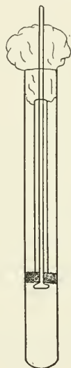
Figure 127. Details of construction of the sponge-and-glass plunger for the collection of cysts. The center rod is solid, and a piece of tubing holds the sponge down.
