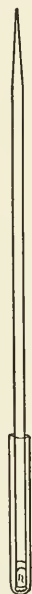
Fig. 124. Migration tube. The tube is filled with a sterile fluid to within about two inches from the top. Protozoa to be sterilized are drawn up under the sterile fluid and the small tip sealed in a flame. The Protozoa migrate upward and are taken off at the top. (Redrawn from Glaser and Coria, 1930.)
