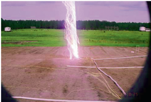
Plate 1 Photographs of lightning flashes triggered at Camp Blanding, Florida. Top – a distant view of a strike to the test runway; middle, a strike to the test power system initiated from the tower launcher; bottom – a strike initiated from the underground launcher at the center of a 70 \times 70 \text{ m}^2 buried metallic grid (See also Figure 2.2 on page 27)
