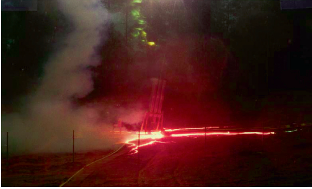
Plate 2 Photograph of ground surface arcing associated with the second stroke (current peak of 30 kA) of flash 9312 triggered at Fort McClellan, Alabama. Lightning channel is outside of field of view. One of the surface arcs approached the right edge of the photograph, a distance of 10 m from the rocket launcher. Adapted from Fisher et al. (1994) (See also Figure 2.12 on page 45)
