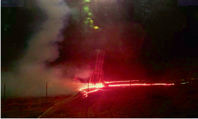
Fig. 2.12 Photograph of ground surface arcing associated with the second stroke (current peak of 30 kA) of flash 9312 triggered at Fort McClellan, Alabama. Lightning channel is outside of field of view. One of the surface arcs approached the right edge of the photograph, a distance of 10 m from the rocket launcher. Adapted from Fisher et al. (1994) (See also Plate 2 in the Color Plate Section on page 594)
