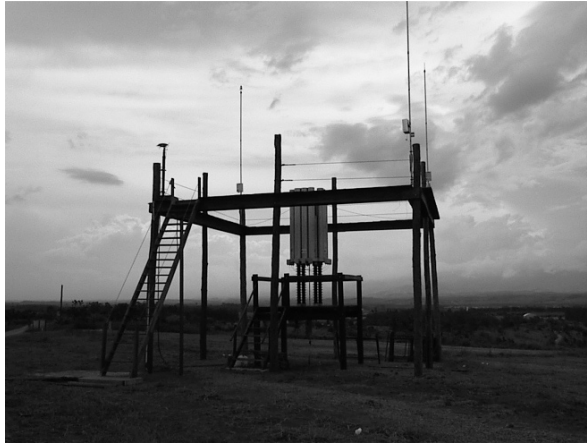
Fig. 9.12 The launching system surrounded by three lightning rods and the control room behind it in the triggering site
