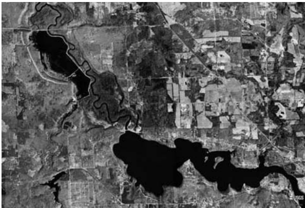
Figure 6 Hydrological alterations to the flood plain along the Kalamazoo River (Michigan USA). This image land is about 11 km in width. The reservoir in the lower part of this view was created by impoundment of the main channel for hydroelectric generation. Downstream is a diked area where water levels are managed for wildlife. The remaining flood plain is covered by deciduous forest and retains an approximately natural flood regime because this and upstream reservoirs do not change seasonally in volume. Image coordinates are 85.94 W, 42.57 N. Image source: U.S. Geological Survey digital aerial photography (DOQQ) taken in March 1999, obtained from NASA World Wind version 1.3.
