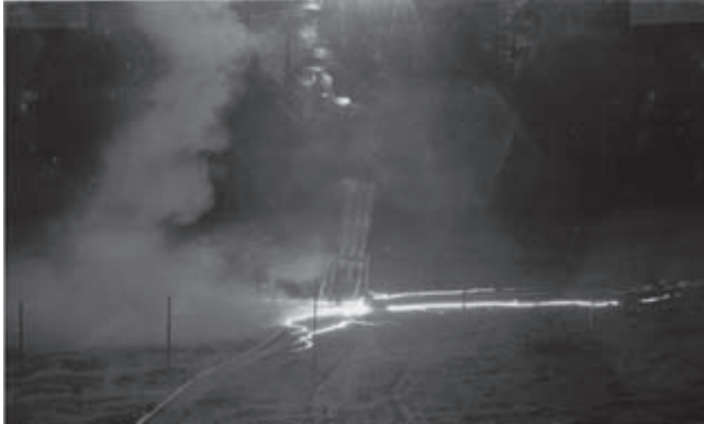
Figure 3.19 Photograph of surface arcing associated with the second stroke (current peak of 30 kA) of flash 9312 triggered at Fort McClellan, Alabama. The lightning channel is outside the field of view. One of the surface arcs approached the right edge of the photograph, a distance of 10 m from the rocket launcher (adapted from Reference 68).
