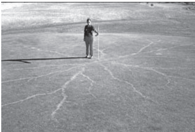
Figure 3.20 Evidence of surface arcing on a golf course green in Arizona (courtesy of E.P. Krider)
