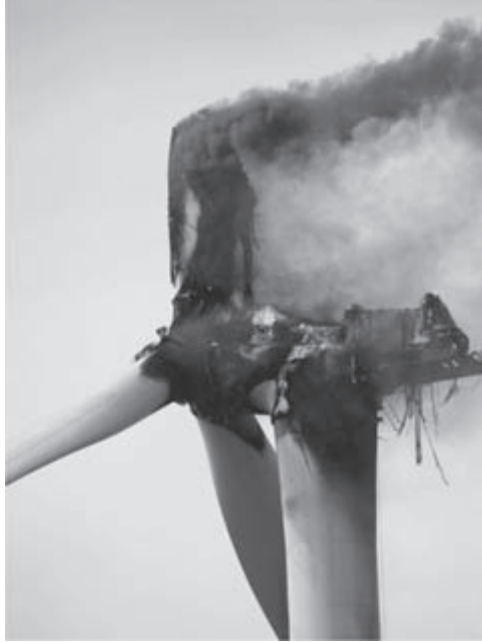
Figure 7.5 Lightning damage at a windpower station
