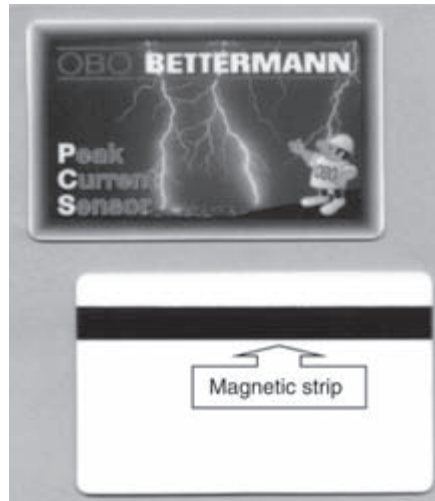
Figure 14.25 Magnetic strip card for registering peak lightning current (photo by the author)
