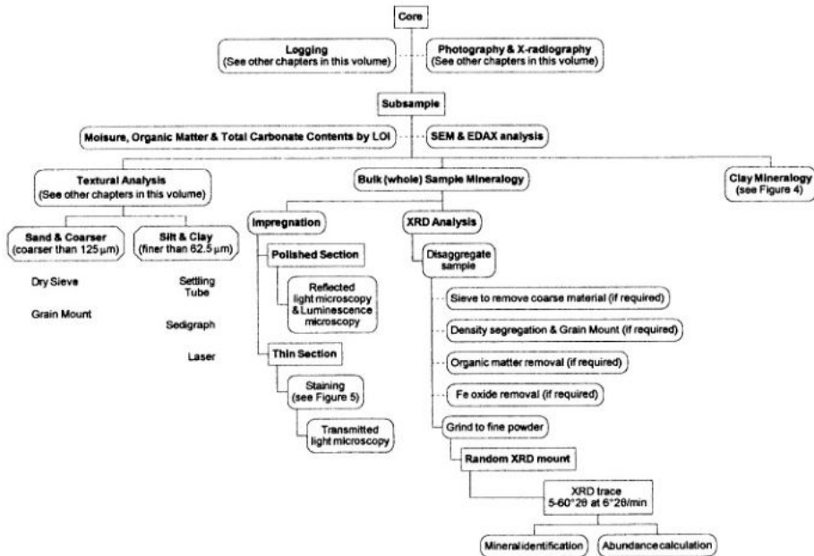
Figure 3. Flowchart showing the usual routes used at University of Manitoba for handling lake sediment samples for mineralogical analyses and other analyses. See Figure 4 for details on the clay mineral (oriented mount) analysis stream.
