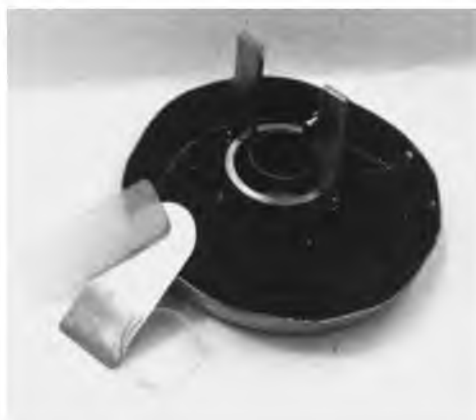
FIGURE 42. Equipment ("frying pan") for subsampling sediment cores with the elimination of the sediment in contact with the core liner.
