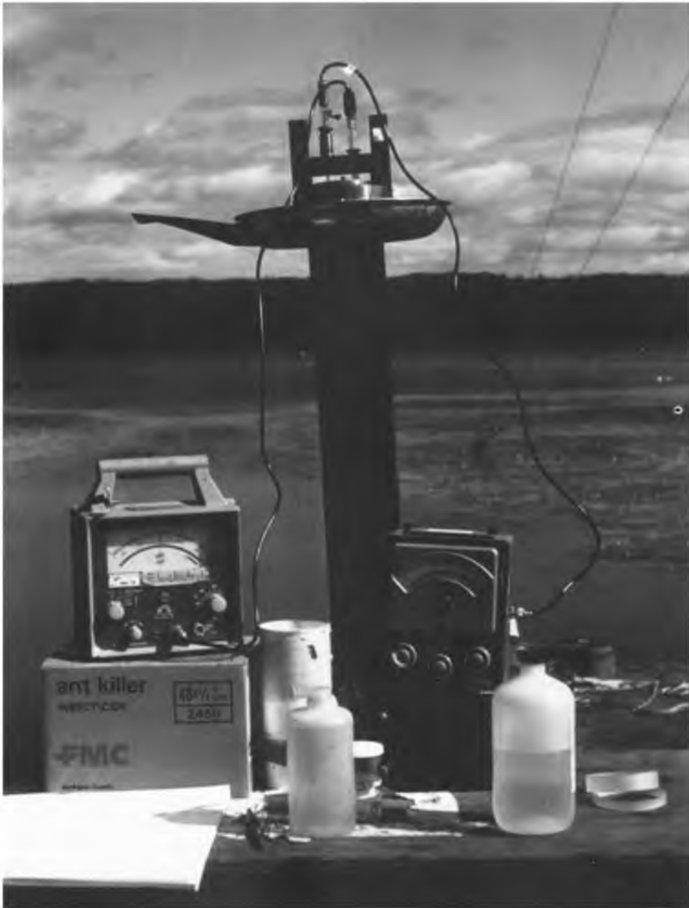
FIGURE 3. Measuring pH and Eh in the field.
