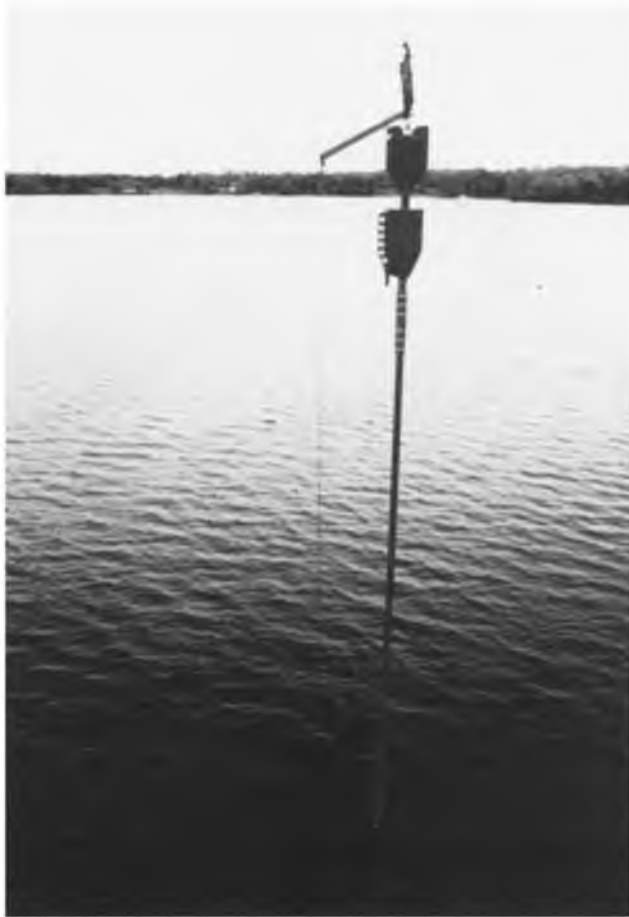
FIGURE 23. Preparation of the piston corer before lowering to the bottom.
