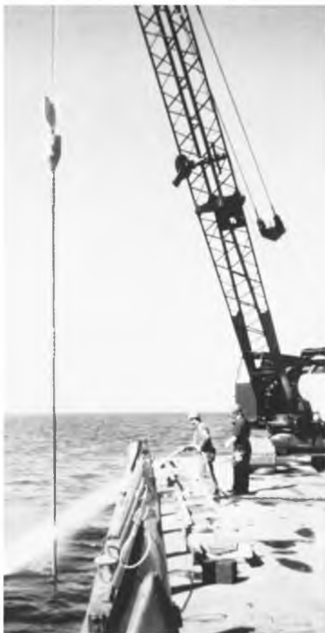
FIGURE 24. Cleaning the piston corer pipes before lifting the corer to the ship deck.
