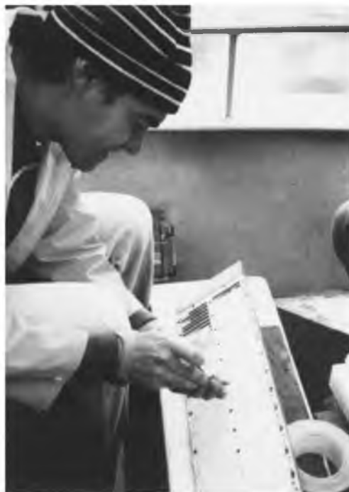
FIGURE 2. Sampling for pore water through the membrane of an in situ dialyzer.
