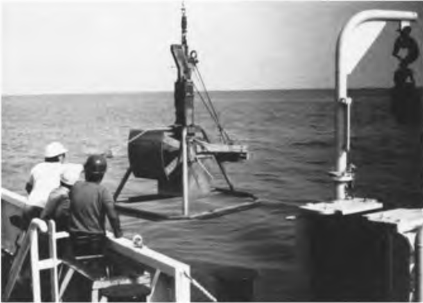
FIGURE 16. Removal of the safety pin prior to the lowering of the box corer to the lake bottom.
