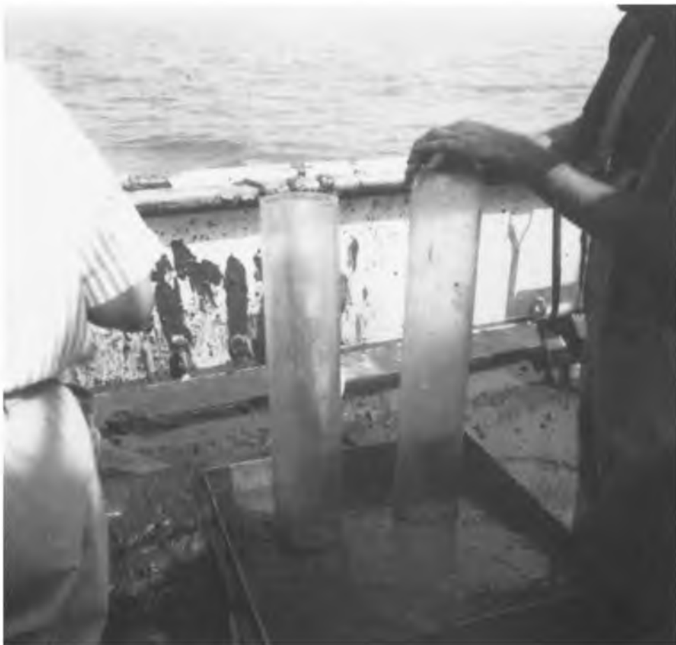
FIGURE 20. Inserting core tubes into the sediment collected by the box corer.
