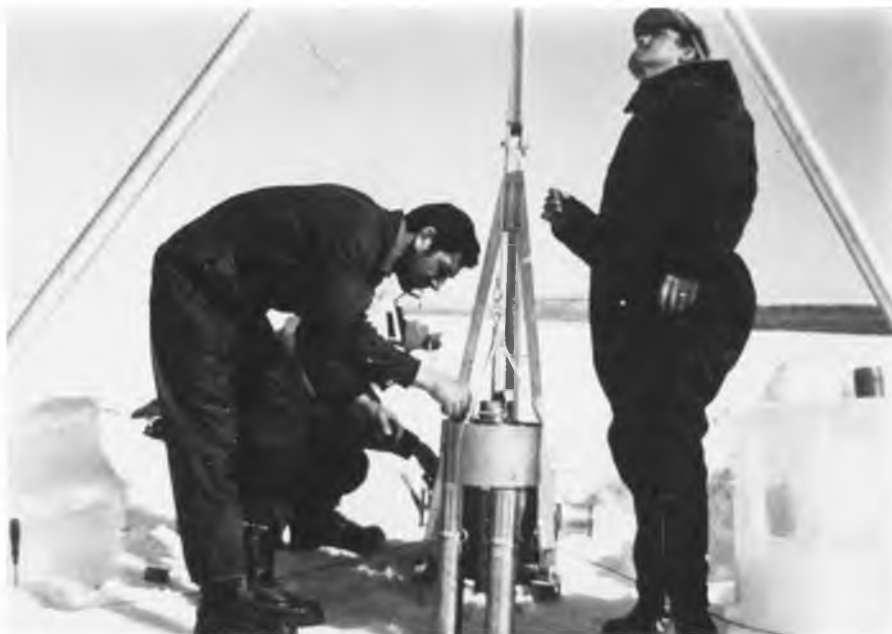
FIGURE 33. Preparation of a multiple corer for sediment sampling from ice.
