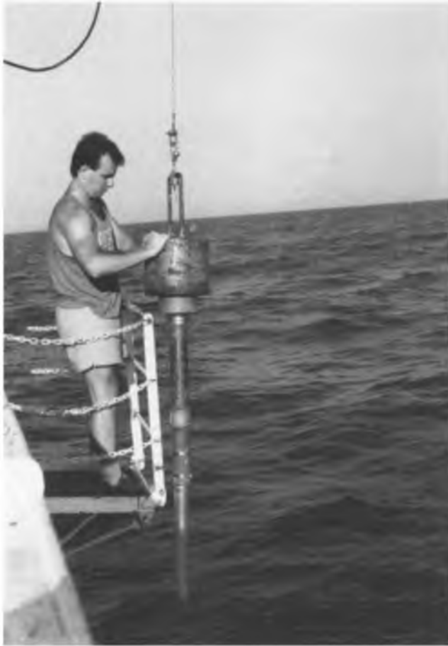
FIGURE 35. Preparation of Benthos gravity corer for sediment sampling.
