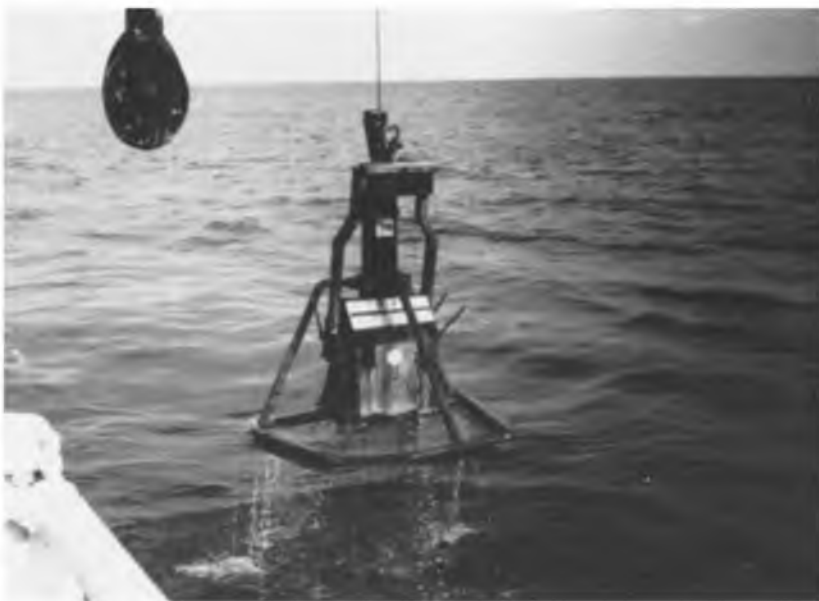
FIGURE 17. Retrieval of the box corer.
