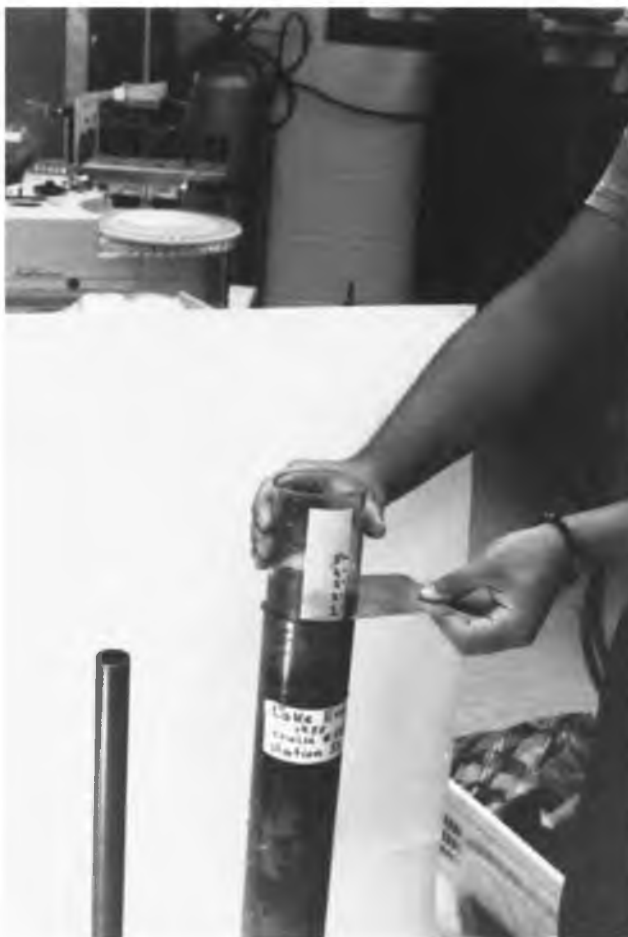
FIGURE 40. Sediment extruded into the piece of core liner with the scale is cut by a metal cutter.
