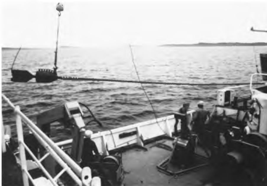
FIGURE 22. Lifting the piston corer before swinging it outboard.
