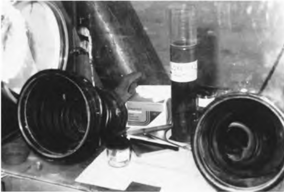
FIGURE 4. Glove box for handling of sediment samples under oxygen-free atmosphere.
