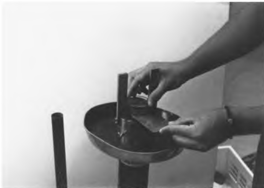
FIGURE 44. Cutting a subsample from the sediment core using the "frying pan".
