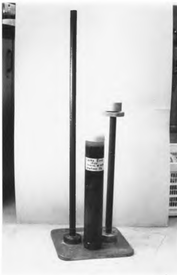
FIGURE 37. Simple piston extruder for subsampling of sediment cores with a metal rod for securing longer cores from falling over, and a labeled sediment core.
