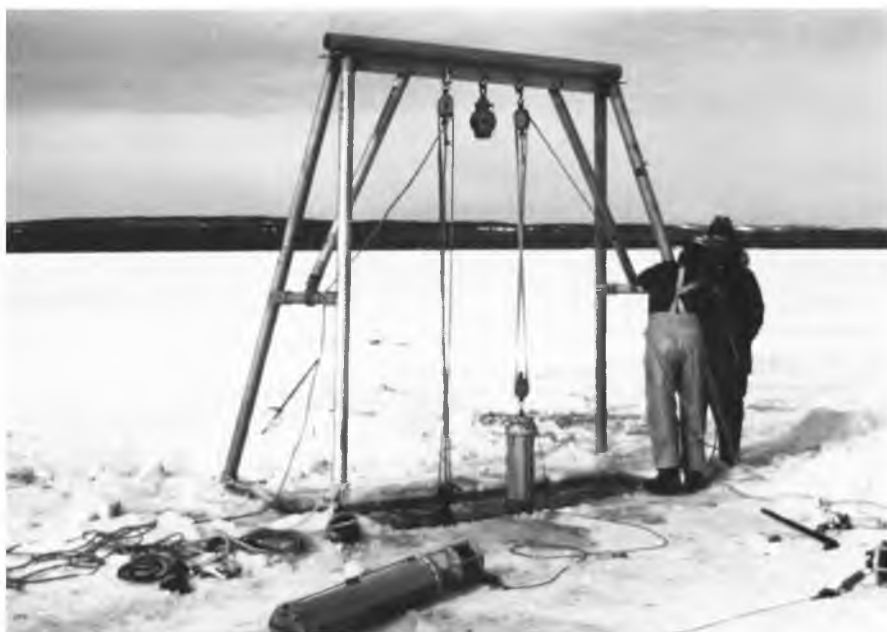
FIGURE 34. Portable frame for lowering the sampling equipment through the hole in the ice.
