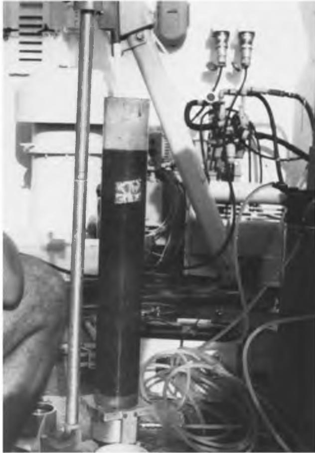
FIGURE 47. Sediment core secured in the extruder.
