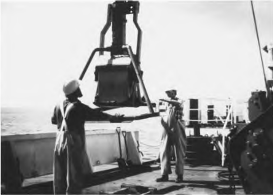
FIGURE 18. Lowering the box corer with sediment to the ship deck.
