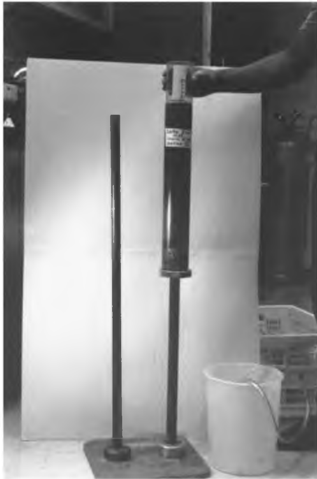
FIGURE 39. Placing a piece of core liner with a scale on the top of the core.
