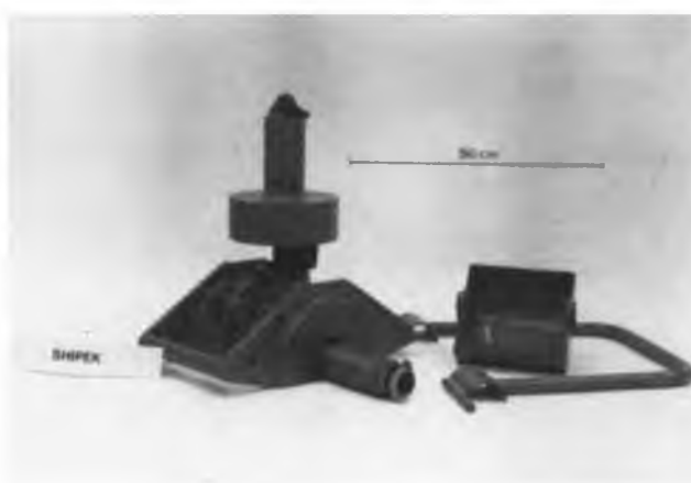
FIGURE 8. Shipek grab sampler with the sampling bucket and cocking lever.
