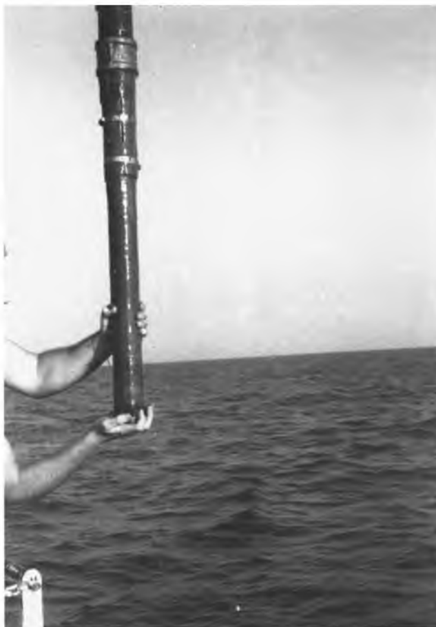
FIGURE 36. Stopping a sediment core collected by Benthos gravity corer.
