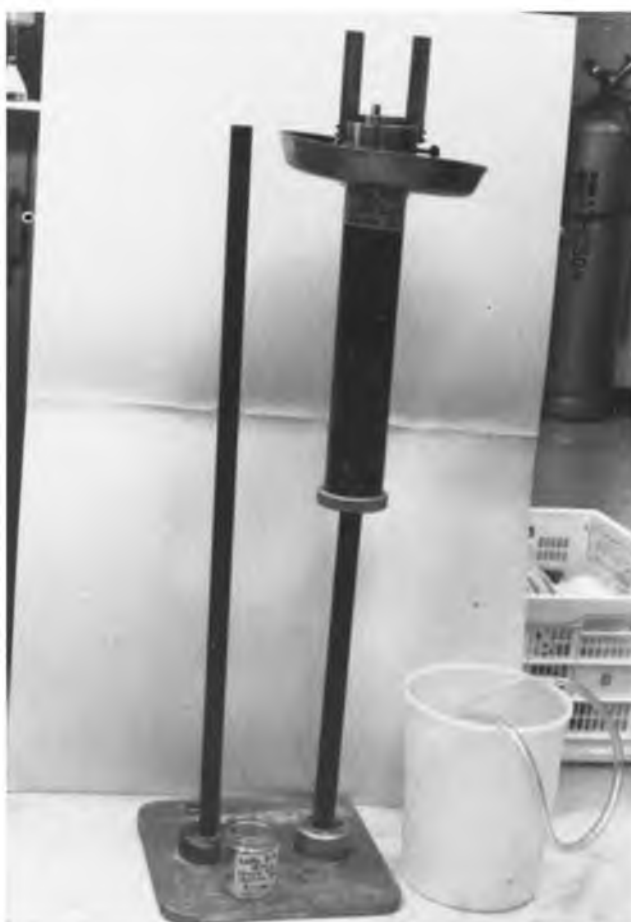
FIGURE 43. "Frying pan" placed on the top of the sediment core before the subsampling.
