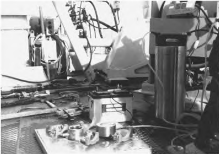
FIGURE 46. Core extruder using pressurized water.
