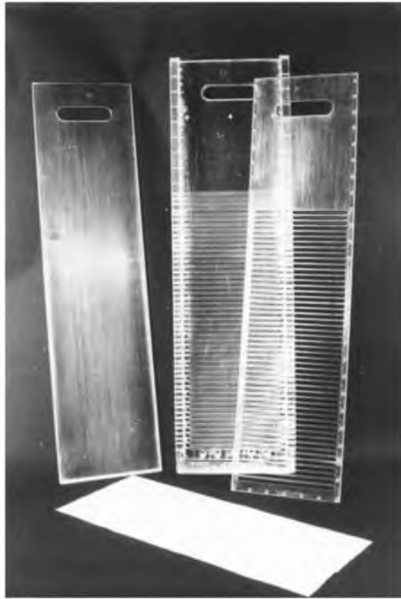
FIGURE 4. An in situ dialyzer with solid cover plate and side ports for removing pore water under an inert gas atmosphere (courtesy of G.Th.M. van Eck).
