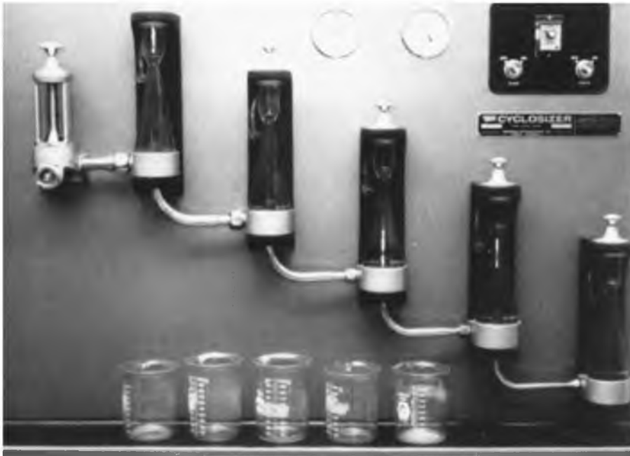
FIGURE 7. Cyclosizer for separation of sediments into different size fractions.
