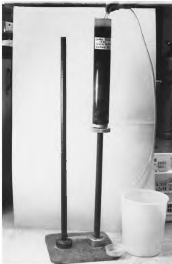
FIGURE 38. Siphoning off the water from a sediment core placed on extruder's piston before starting the subsampling.
