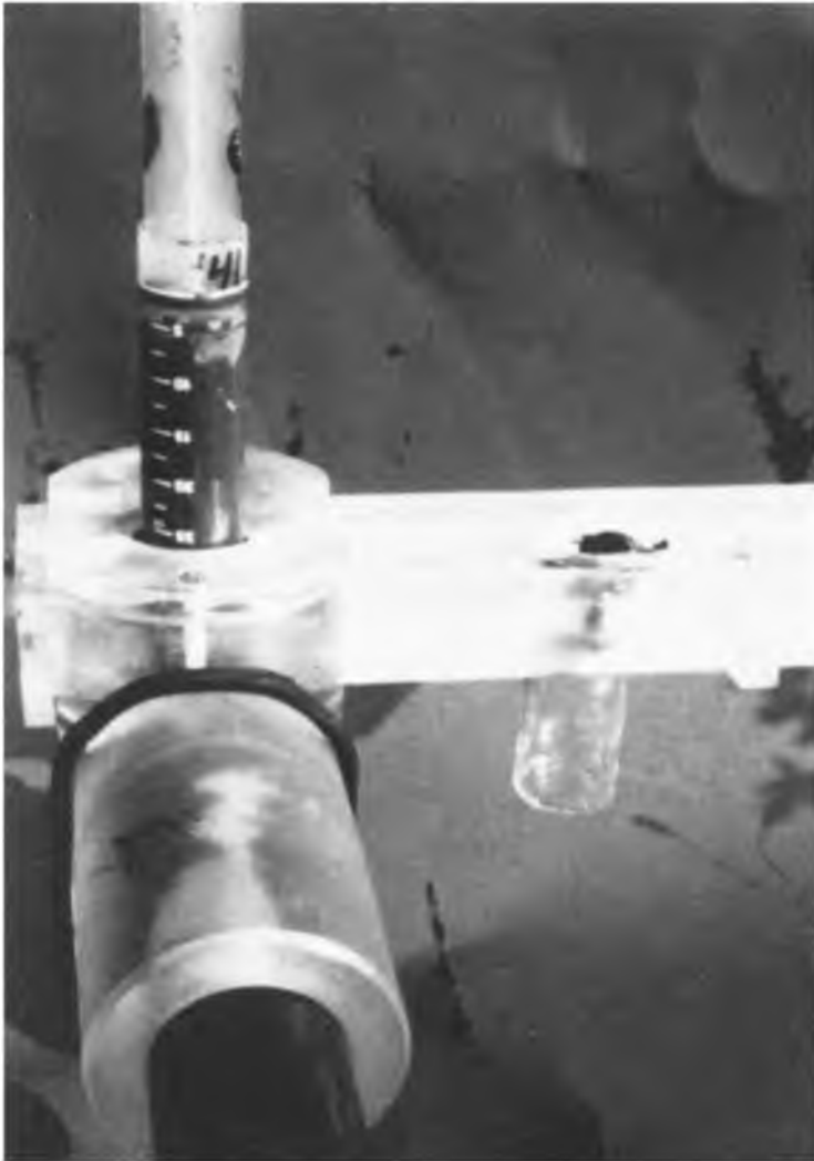
FIGURE 6. The core adapter syringe sampling (CASS) system to collect sediments for gases, including 4-cm o.d. sediment core and top plastic slider containing filled 25-ml serum monovette plastic syringe, empty scintillation vial (for determination of water content), and syringe cap (illustrated from left to right).
