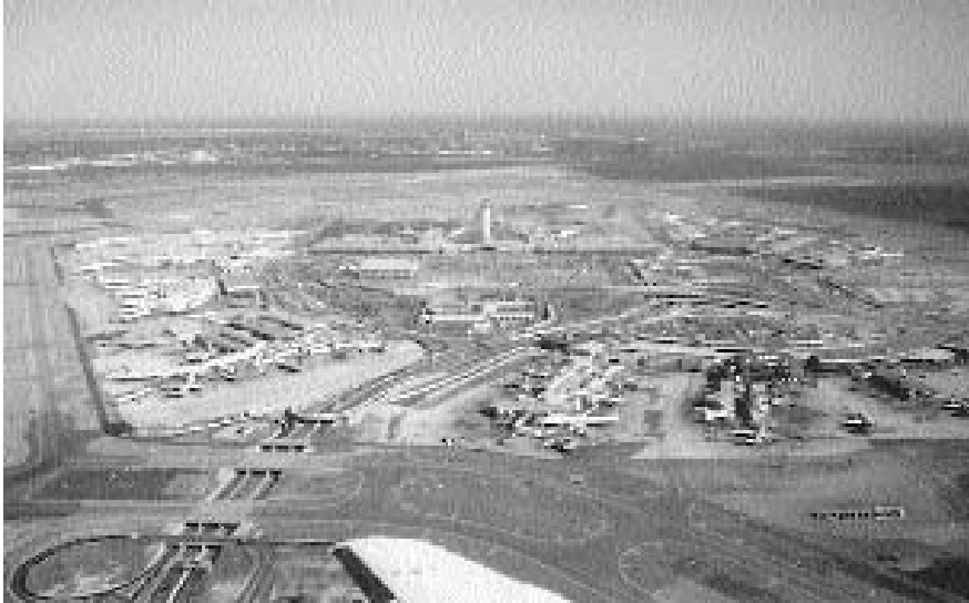
Figure 6-3. JFK International Airport in New York City provides an example of a multiple-unit terminal concept. (Source: www.airliners.net)
