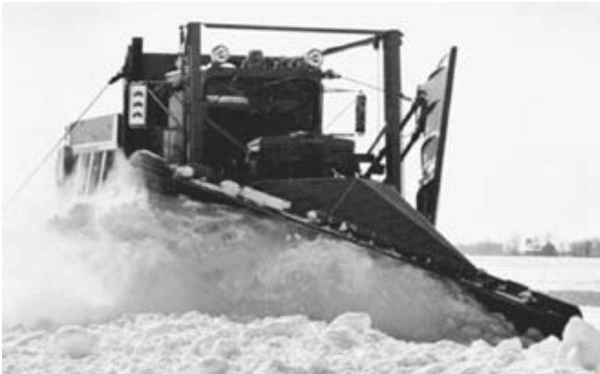
Figure 7-4. Snowplows move the snow to the pavement edges where snowblowers disperse the windrowed snow. (Photo courtesy FAA)
