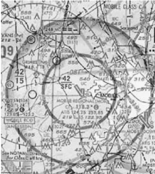
Figure 5-7. Class C airspace surrounding Mobile, Alabama, International Airport. (Source: National Aeronautical Charting
