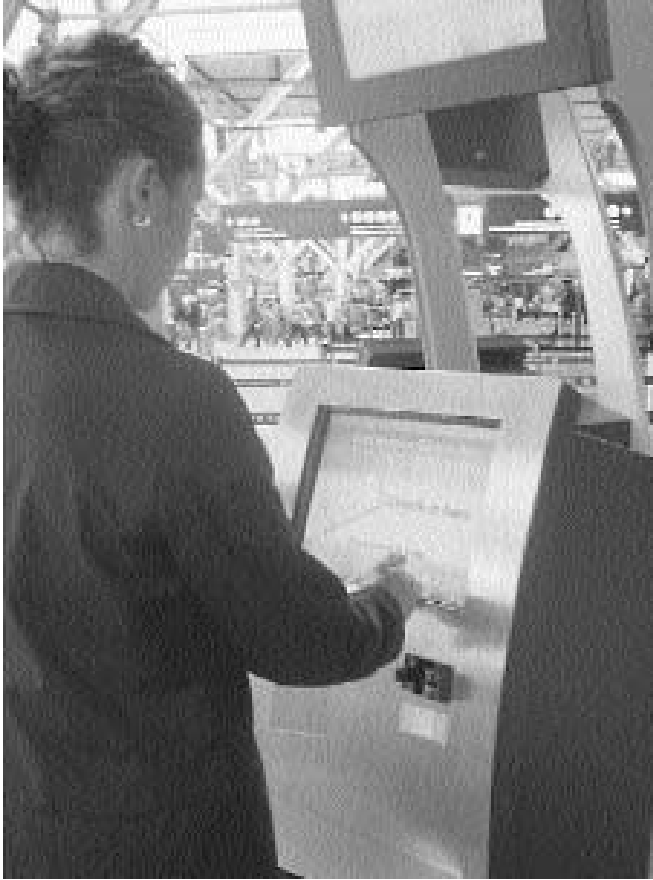
Figure 6-17. Common use self-service (CUSS) kiosk.
