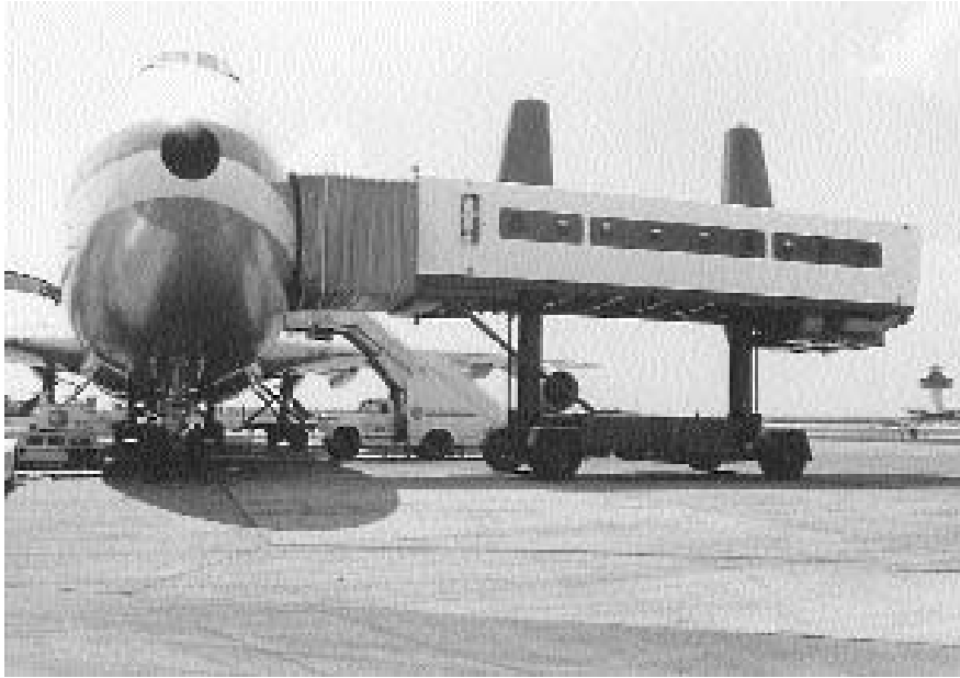
Figure 6-9. Mobile lounge attached to aircraft at Washington's Dulles International Airport, circa 1970. (Photo courtesy Metropolitan Washington Airports Authority)
