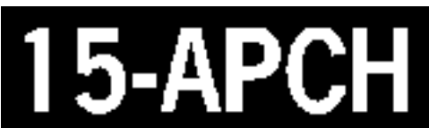
Figure 4-26. Runway approach area holding sign. (Source: FAA AIM)
