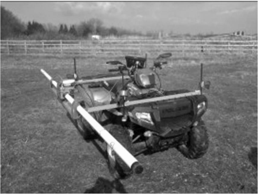
**Figure 1.16** *Geonics EM-31 mounted on a quad bike. Induced currents will flow in the vehicle as well as in the ground, but should be reasonably constant.*
