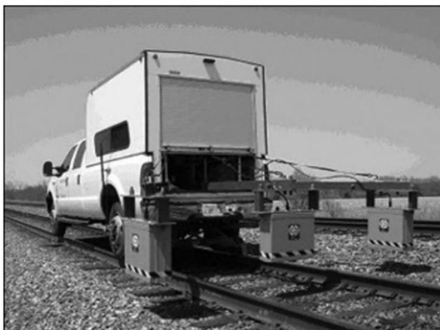
**Figure 10.14** Radar system with air-launched horn antennas being used to monitor railway trackbed ballast.
