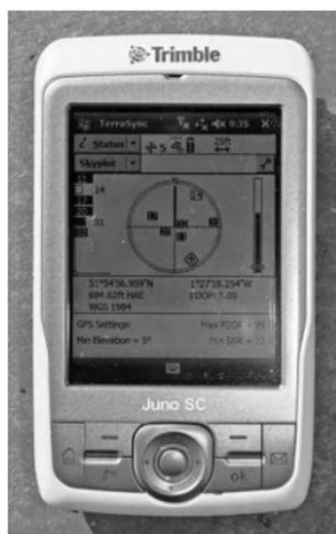
**Figure 15.1** Example of a hand-held Personal Digital Assistant (PDA) and global positioning system (GPS) receiver that can receive real-time differential GPS (DGPS) corrections via satellite to provide 2–5 m locational accuracies. It is equipped with WiFi and Bluetooth for easy email and data exchange.
