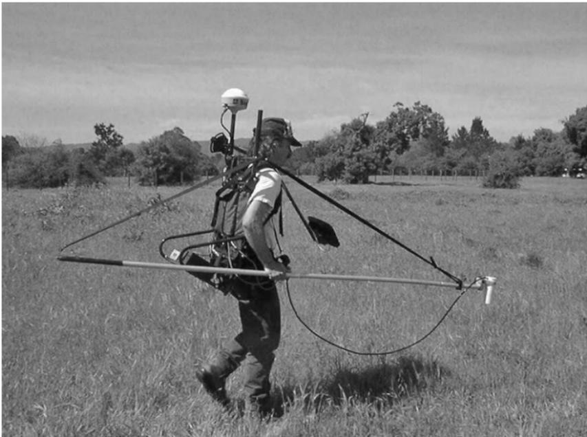
**Figure 1.15** Magnetometer coupled to a differential GPS navigation system for continuous profiling. Unless allowance is made in processing for the offset between the GPS and magnetic sensors, anomaly locations will be incorrectly plotted (photo courtesy of Geometrics).
