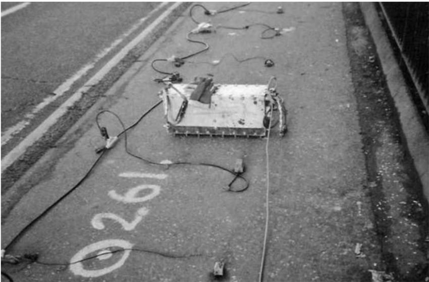
*Figure 12.9* MicroVib shear-wave (SH) reflection source.
