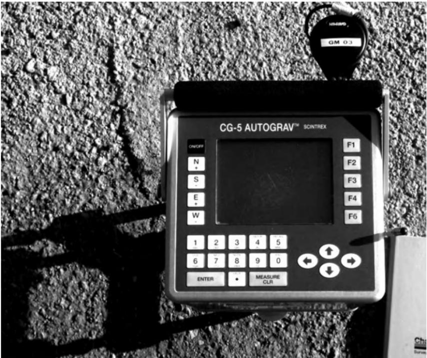
*Figure 2.4 The Scintrex CG-5 automatic gravity meter.*
