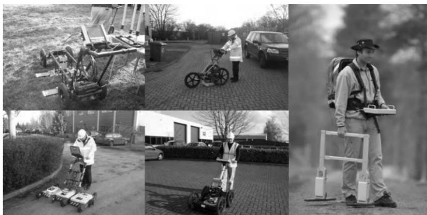
**Figure 10.13** Examples of commonly available radar systems utilising ground-coupled dipole or bow-tie antennas.
