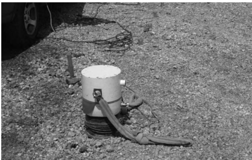
*Figure 11.5* Electromagnetic vibrator source.
