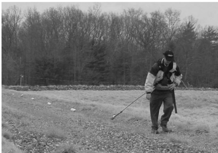
**Figure 6.14** Towing the OhmMapper™. Photo reproduced courtesy of Geometrics Inc.
