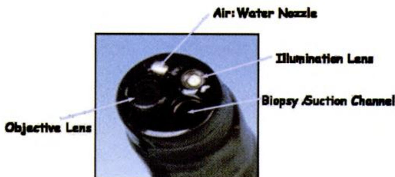
Figure 2-3. End view of the distal tip of a forward Olympus fiberscope.
