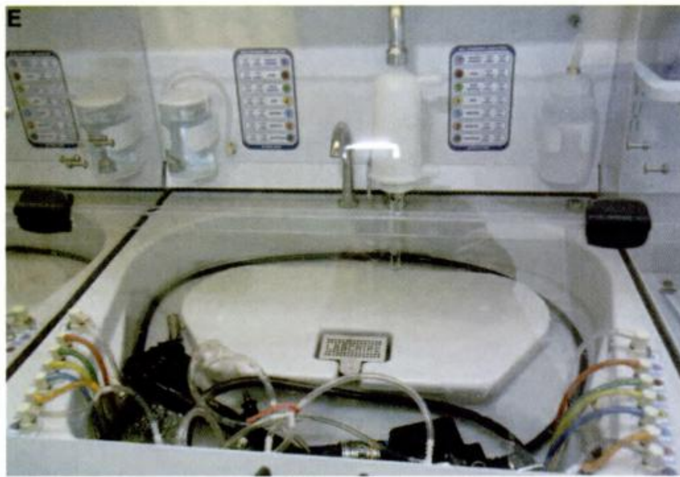
Figure 4-9. Continued Using the automated washer disinfector to clean the endoscope.
