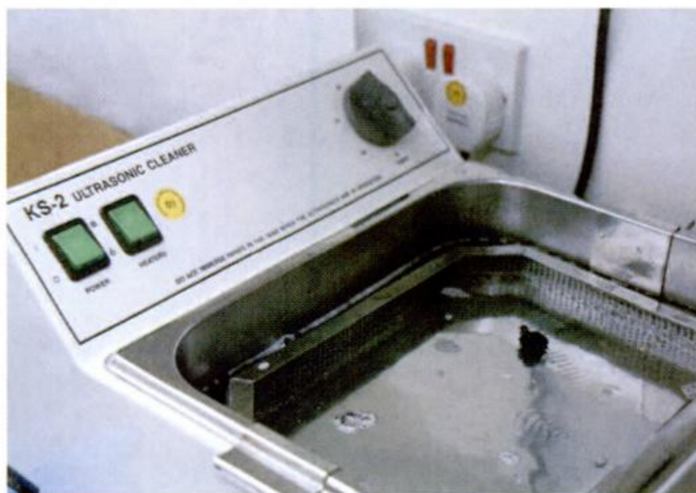
Figure 4-10. Ultrasonic cleaning of endoscopic equipment prior to disinfection.
