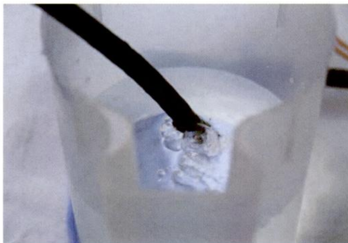
Figure 7-3. Checking that air insufflation is satisfactory.
