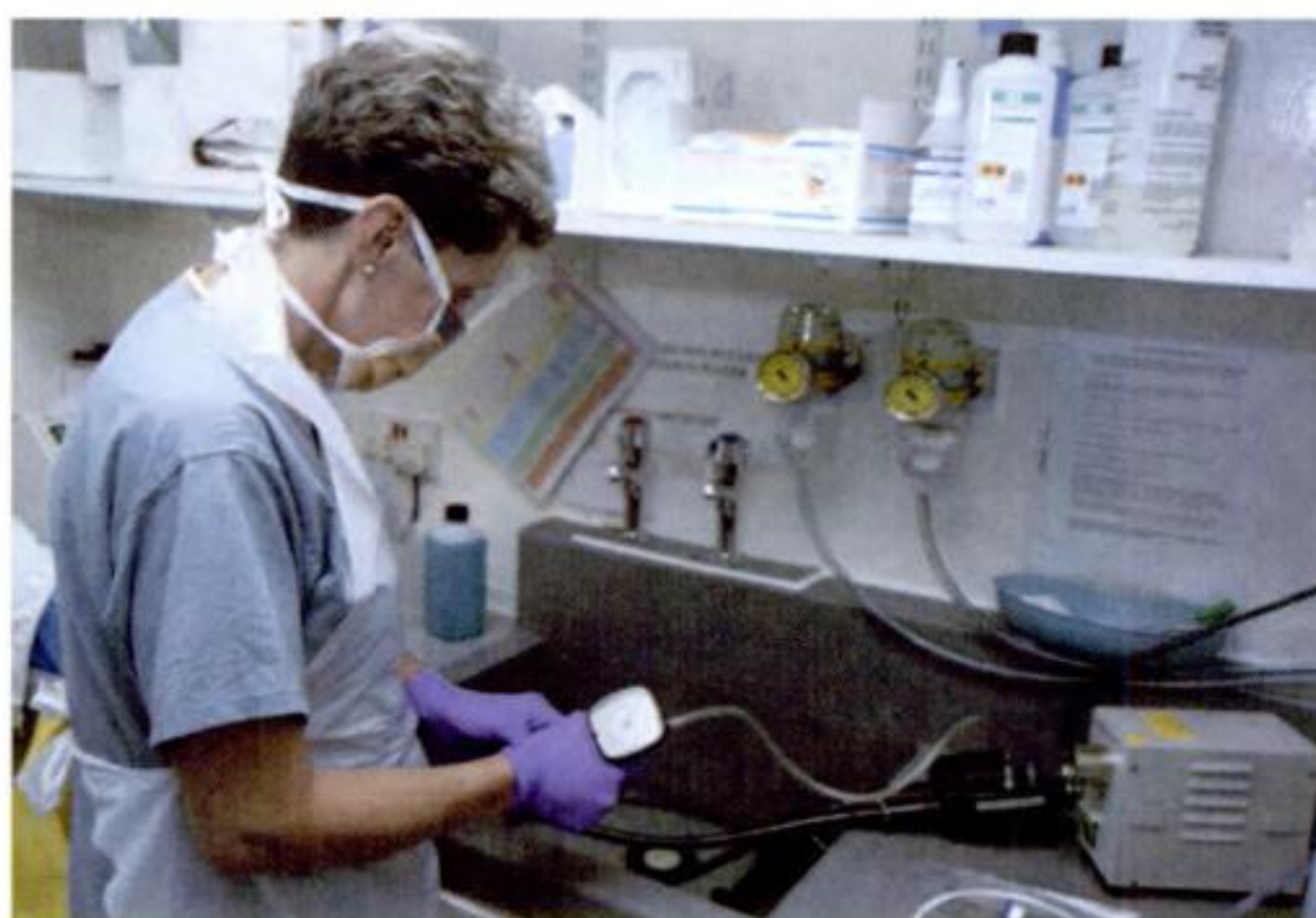
Figure 4-3. Leak testing of endoscope prior to submersion.
