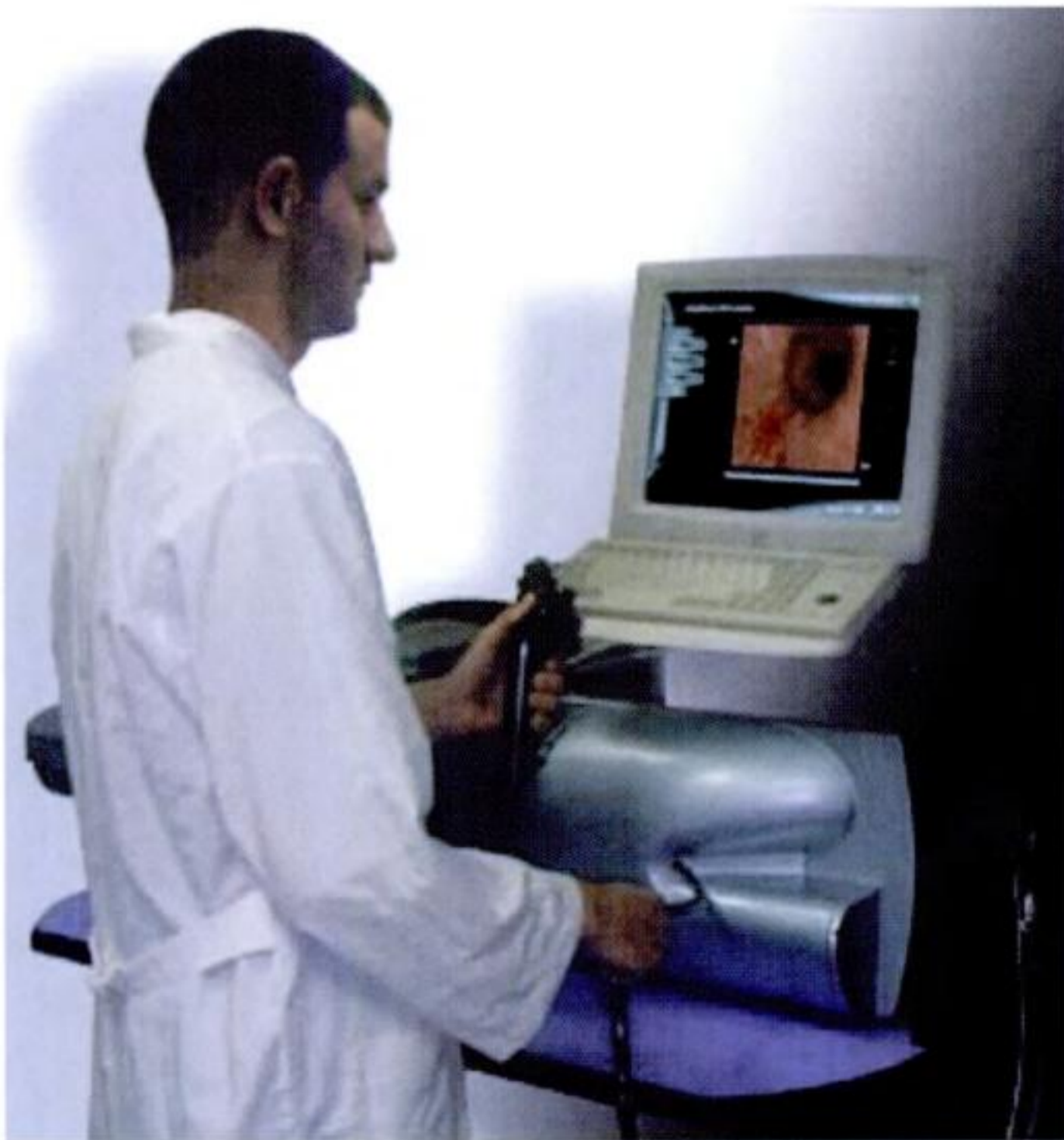
Figure 3-4. Symbionix GI-Mentor simulator being used for training in upper gastrointestinal endoscopy and colonoscopy.
