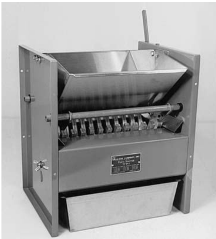
FIG. 10.8 A Jones sample splitter. For explanation see text.
