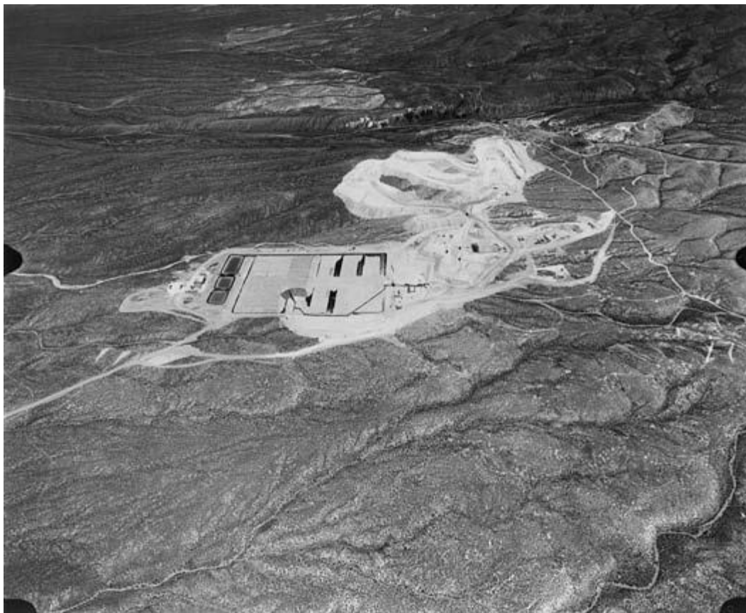
FIG. 16.7 Aerial photograph of Trinity Mine. The light areas in the center represent waste and low grade ore stockpiles. The medium tone areas in the foreground show the extent of the alteration in the area. The rectangular area is the heap on which the ore is placed for cyanide leaching. The ponds in which the pregnant solutions collect are seen next to the mine buildings. (Photograph supplied by US Borax.)
