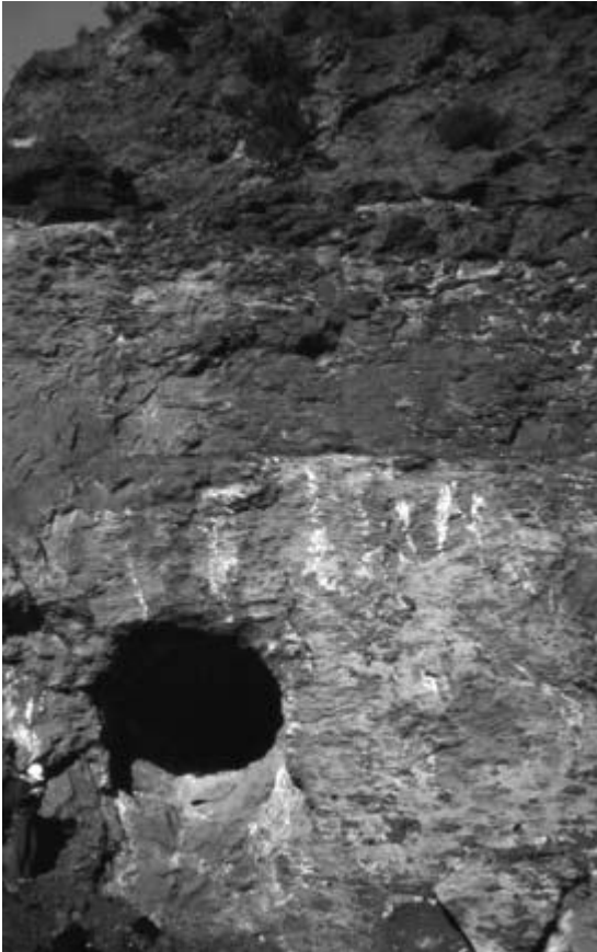
FIG. 5.4 Gossan (above adit) overlying sulfides exposed in the pit wall of the San Miguel deposit, Rio Tinto, southern Spain.
