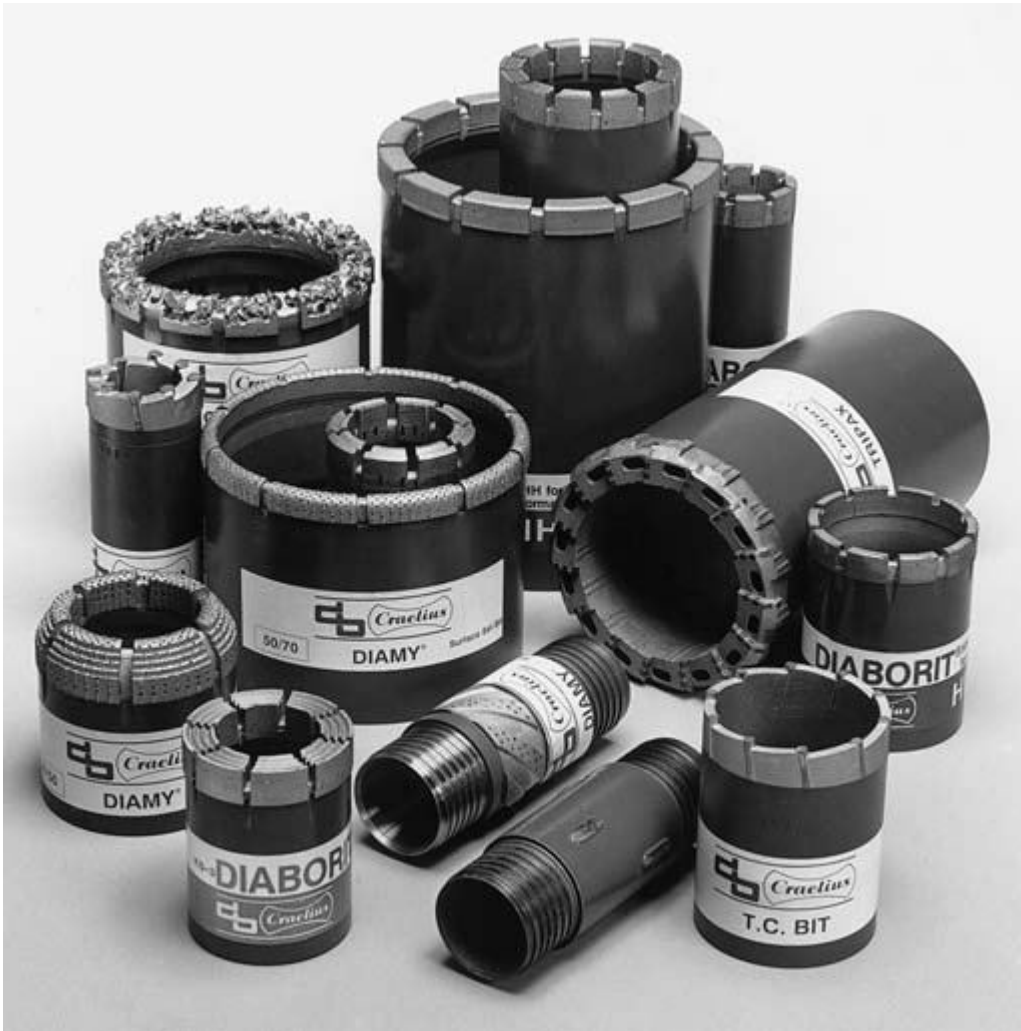
FIG. 10.11 On the left-hand side are several types of surface-set diamond bits, on the right are bits with tungsten carbide insets and at the back are impregnated bits. (Reproduced by permission of Diamond Boart Craelius Ltd.)
