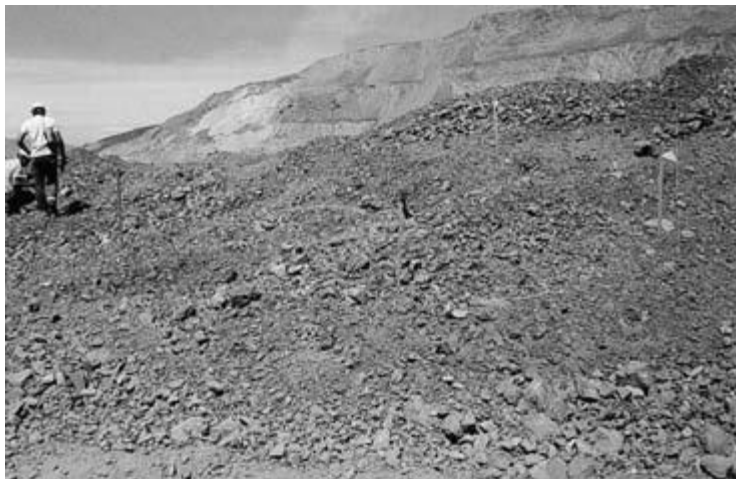
FIG. 16.8 Photograph showing the color-coded flags used to delineate ore from waste in the pit. The dark flags denote ore blocks and the pale flags denote waste blocks.
