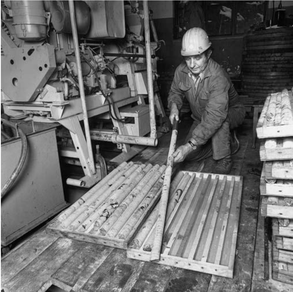
FIG. 10.13 Diamond drill core being examined and stored in a wooden core box. Note the excellent core recovery. (Reproduced by permission of Diamond Boart Craelius Ltd.)
