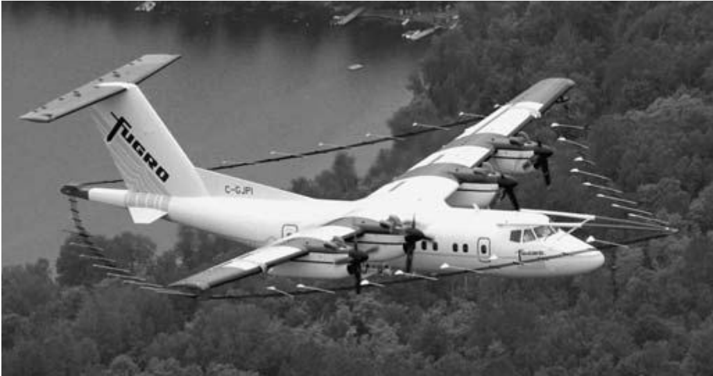
FIG. 7.2 Airborne geophysical installation. The aircraft has been modified for combined magnetic and TEM surveys. The boom projecting from above the cockpit is the forward mounting of the electromagnetic transmitter loop, which extends from there to the wingtips and then to the tail assembly. The magnetometer sensor is housed in the fibreglass "stinger" at the rear, which places it as far as possible from magnetic sources in the aircraft.
