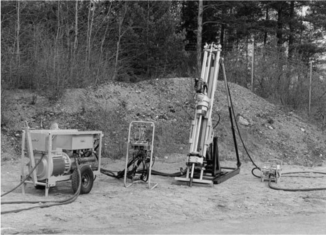
FIG. 10.10 A diamond drill. From left to right the components are the power, control, drill, and water pump units. (Reproduced by permission of Diamond Boart Craelius Ltd.)
