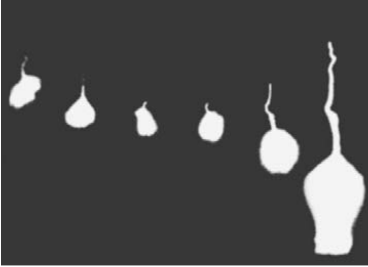
Figure 3.46 Successive frames of image converter picture in a 10 m gap showing the development of streamer discharges from the head of the leader channel [60]
