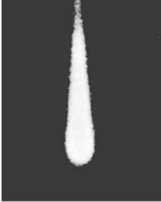
Figure 3.8 Cloud chamber photograph of a single electron avalanche (from [62])
