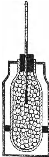
FIG. 243. Apparatus to show that Heat is liberated in Respiration.
